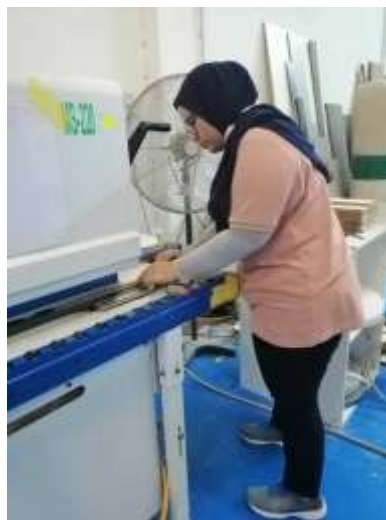
Figure 4. The edging process using the edging machine
