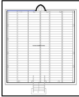
Figure 14. KTTM Floor Plan. This rectangular floor plan is designed without a column structure in the middle that supports the load from the roof structure. Looks like a curved-shaped mihrab on the forefront of the imam's use in congregation prayers.
