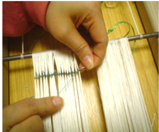
Figure 17: Tying of weft yarns using raffia according to the design given. (Source: Norwani Md. Nawawi, 2003)
