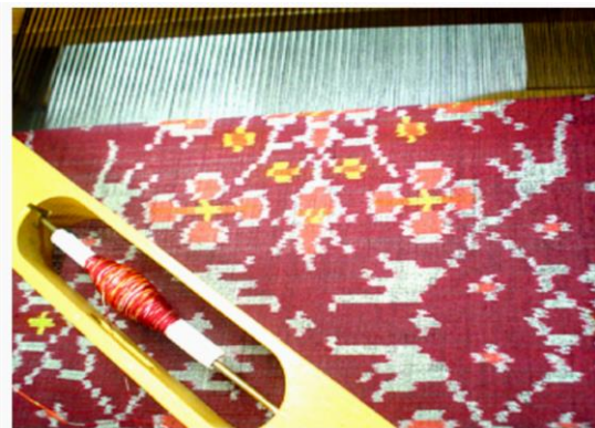
Figure 20: In weaving ikat limar , each weft thread woven must be registered according to the design given. (Source: Norwani Md. Nawawi, 2003)
