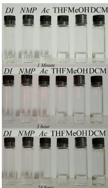
Figure 6. Digital picture of N 3 -PMeOxz solubility in solvent. Top: After 1 min. Middle: After 3 h. Bottom: After 24 h.
