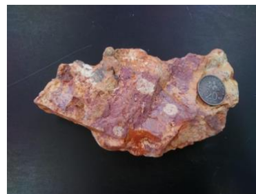
Figure 5. Hand specimen of weathered greywacke sandstone, contain clay clasts.
