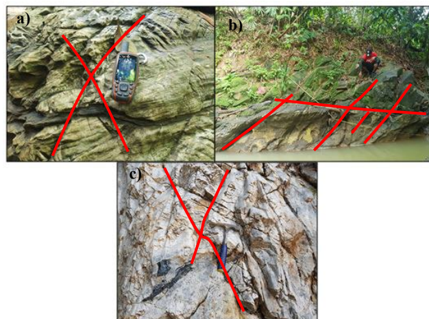
Figure 3: a), b) Example of conjugate shear joint exposed on the outcrop and c) similar shear joint orientation found in the field.
