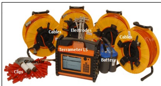
Figure 4: Equipment used for resistivity survey.
