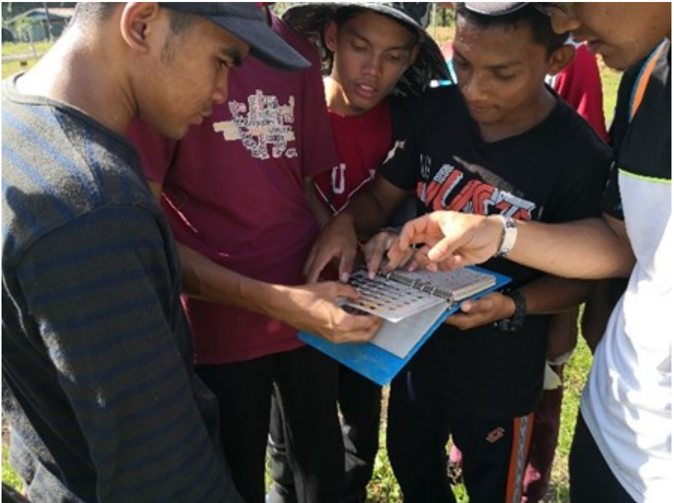
Observing soil colour using the Munsell Chart
