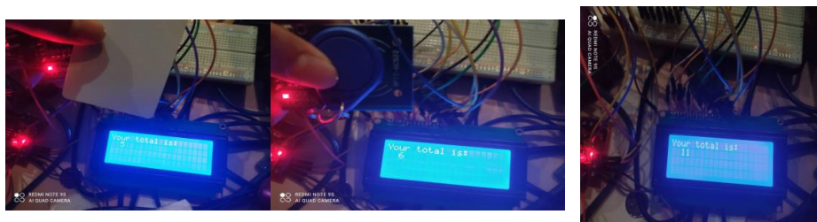
Figure 5. LCD outcome upon RFID tags detection
