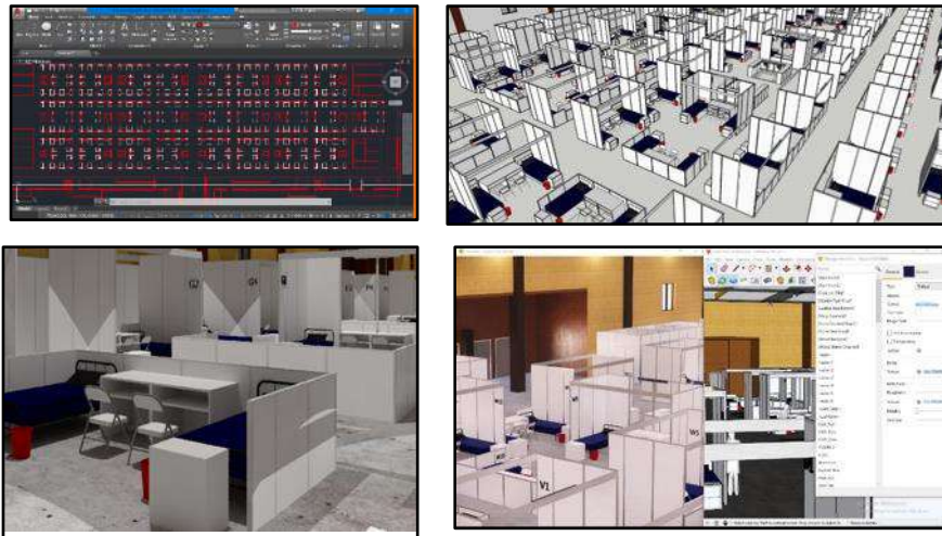
Figure 2: Developing 3D animation of PKRC hall of MAEPS using AutoCAD, Sketch Up and V-Ray
