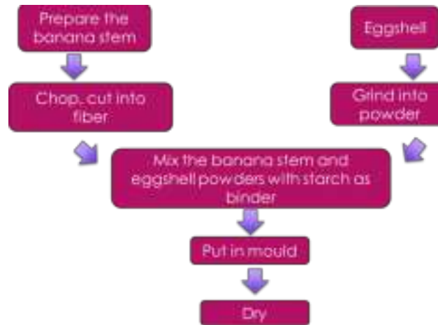
Figure 1. The overview of BioG Pot preparation.
