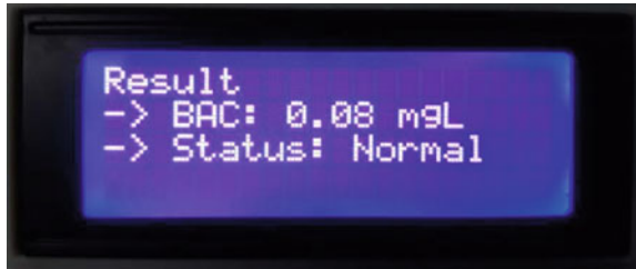
Fig. 9 The Blood alcohol level (BAC) will be displayed on LCD to show the alcohol status of the user
