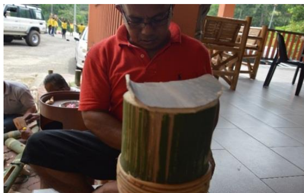
Figure 16. Measure the area of the upih to insert a small part of the upih into the bamboo
