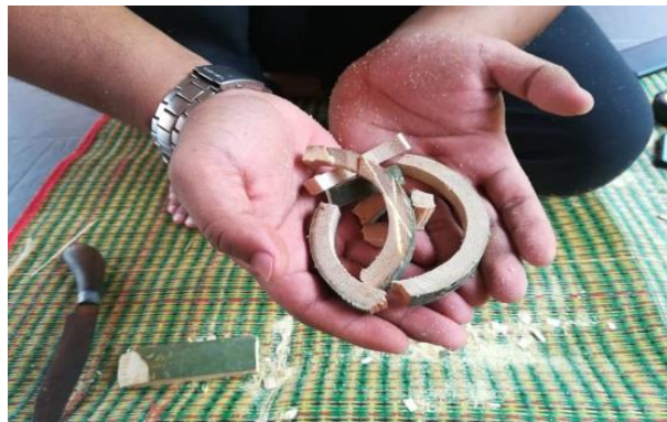
Figure 13. Excess bamboo is cut to make a stopper
