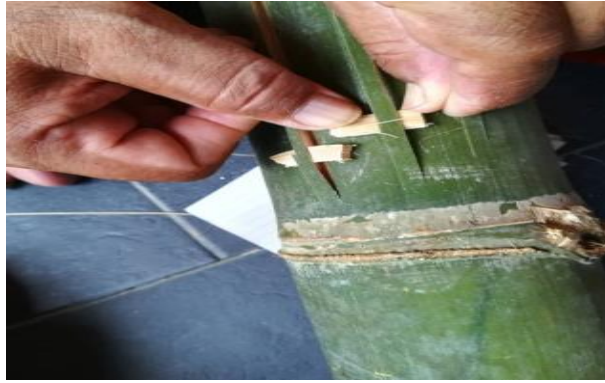
Figure 14. Insert the stopper on the bamboo rope to find a better sound
