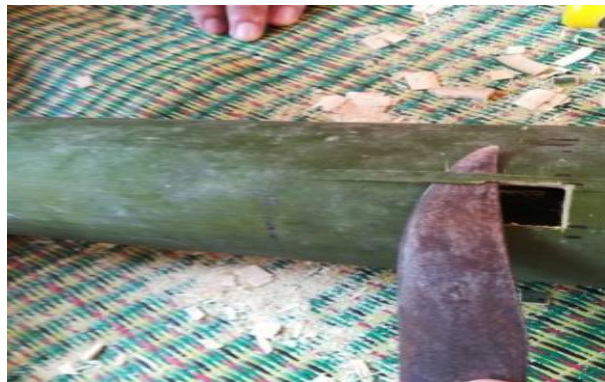
Figure 10. Dig a little part of the bamboo to make a bamboo rope
