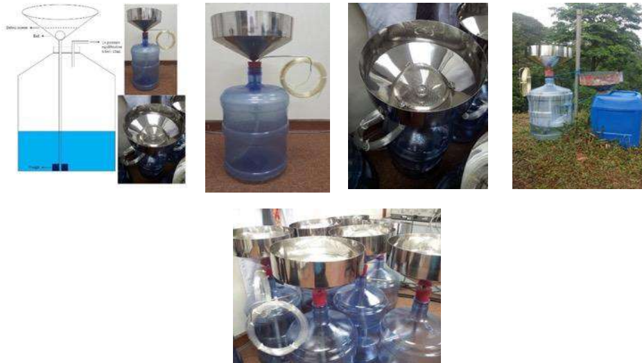
Figure 1: Above pictures showing setup of rainfall collector
