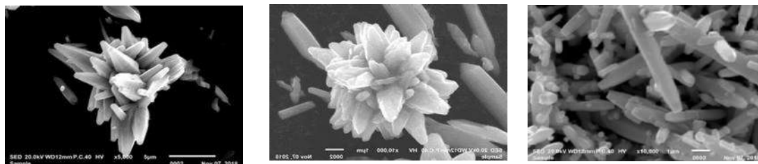
Figure 2.0: SEM image of ZnO nanostructures prepared at different pH values
