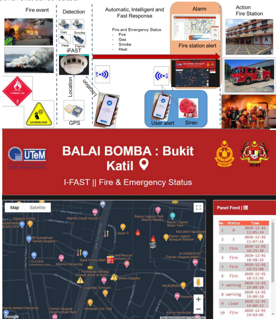
Figure 1 Developed hardware and software for IFAST
