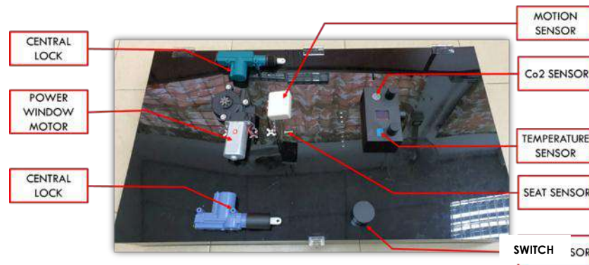
Figure 2 : Integrated between VAS and car's system
