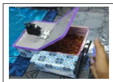
Figure 1 (c) Prototype of Low-Cost Automatic Cat Feeder
