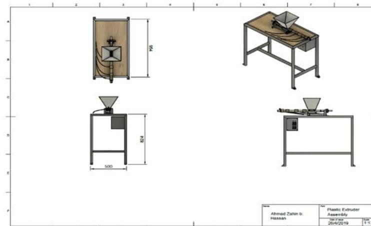
Fig 2. Technical Drawing of Extruder Design
