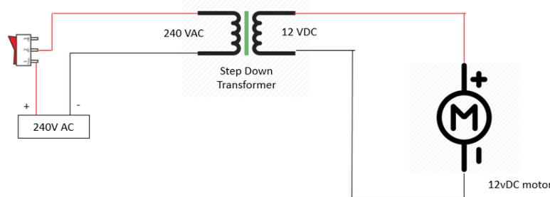
Fig. 6: Schematic Diagram for Motor
