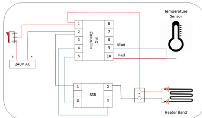
Fig. 5: Schematic Diagram of Heating Element
