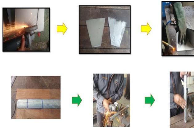
Fig. 3: Hopper and Barrel Fabrication Process
