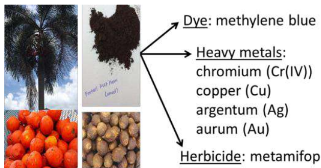
Figure 1: The activated carbon from foxtail palm fruit that applied in adsorbing various types of pollutants such as herbiced, dye and heavy metals
