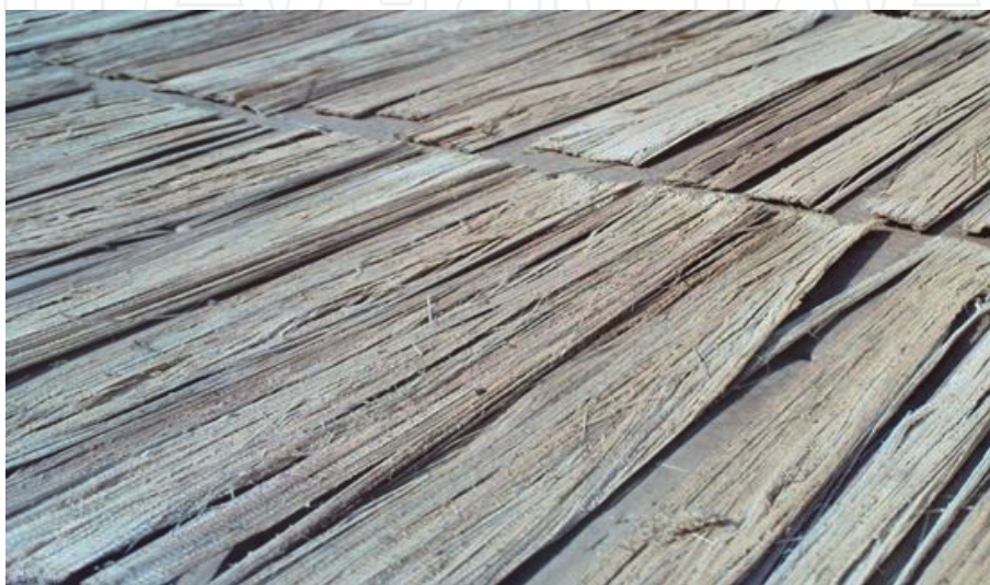
Figure 18. Compressed oil palm fronds under sun-drying.
