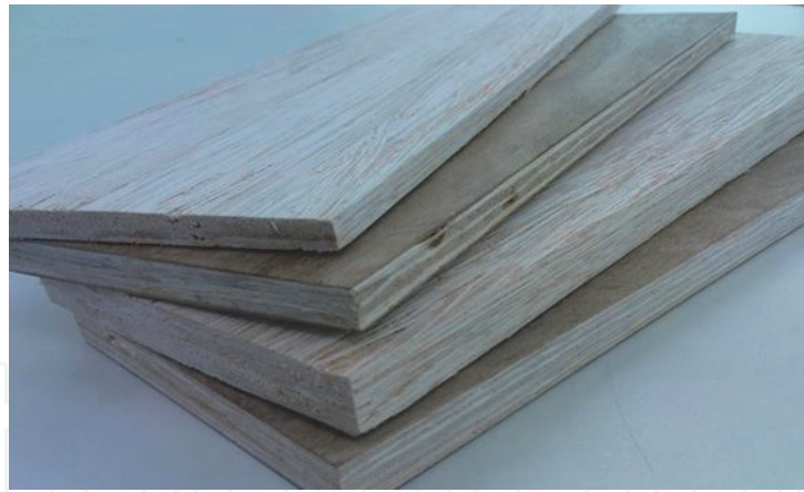
Figure 23. The compressed oil palm fronds boards at differences thickness.
