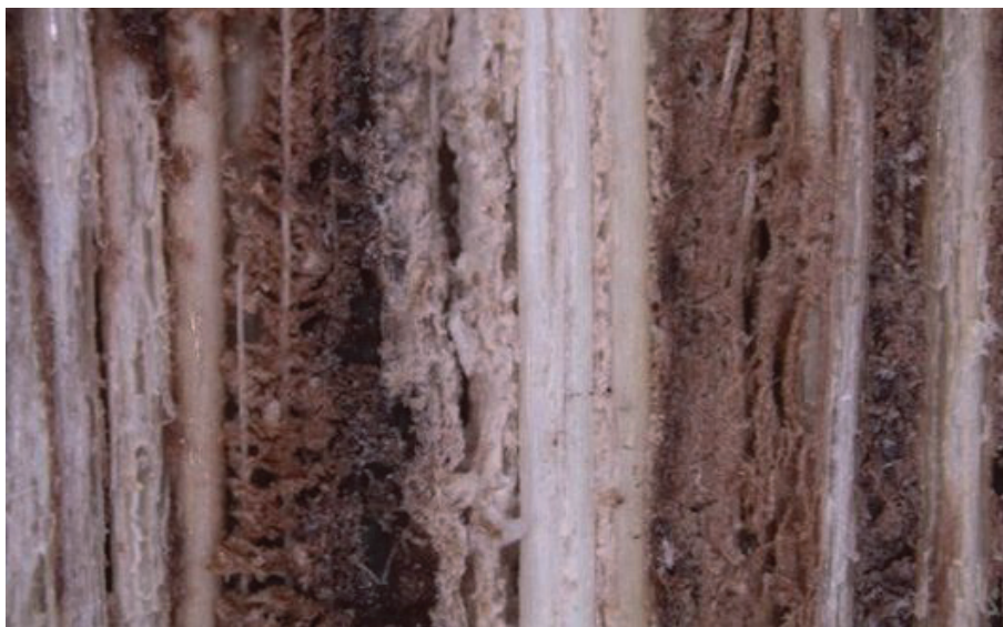
Figure 24. High-performance micrograph of the phenol-formaldehyde composite board from compressed oil palm fronds at the longitudinal sectional view (2× magnification).
