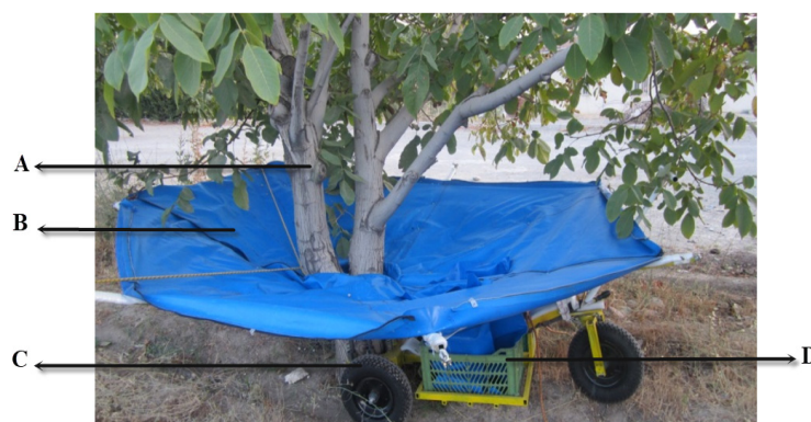
Figure 8. Collector system parts. (A) Tree trunk. (B) Polyester cover. (C) Wheels. (D) Box.
