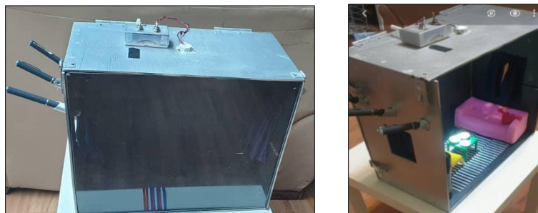
Figure 1. Nur Mobile Lab is a lighting box to demonstrate lighting principles
