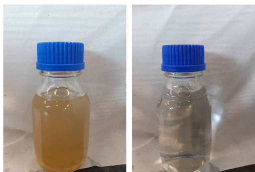
Fig. 8. Appearance of the raw groundwater. (a) before treatment (26 NTU) and (b) after treatment with MBAC (0.4 NTU)
