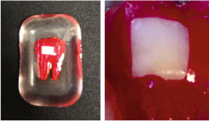
Fig. 1 Tooth sample was colored with red nail polish leaving a 4 mm × 4 mm square window (right). The tooth sample was molded into epoxy resin for positioning, inducing of caries and scanning under the OCT (left)
