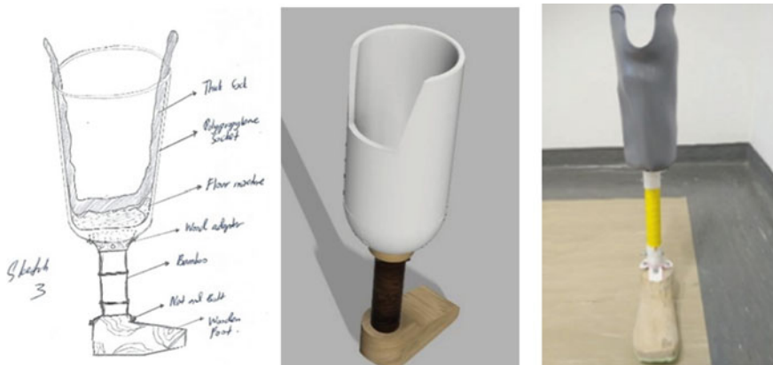
Fig. 1 Design sketch of the interim prosthesis (left), 3D drawing (middle) and completed prototype (right)
