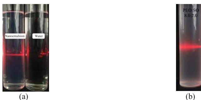
FIGURE 4. Tyndall effect test on nanoemulsion, and distilled water (a) and Tyndall effect on nanoemulsion containing Piper betle essential oil (b)
