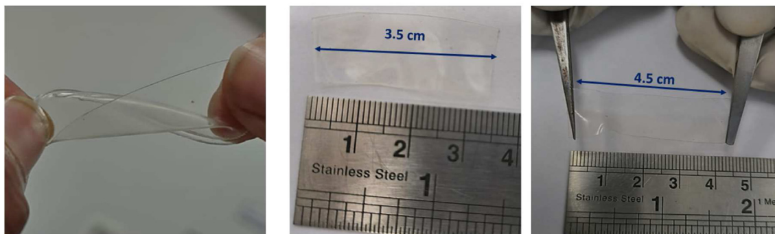
Fig. 2. Highly flexible Ionic liquid doped solid polymer electrolyte (ILDPE) films.
