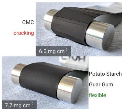
**Figure 6.** The bending test of CMC and potato starch [171]. Adapted with permission from Ref. [171] (Copyright 2020, Wiley).
