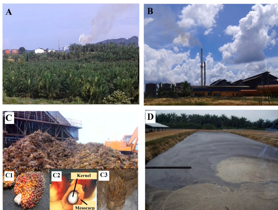
Fig. 2. A) Typical oil palm plantation with palm oil mill; B) Palm Oil Mill; C) Piles of Oil Palm Empty Fruit Bunches waiting to be transported, C1: Fresh Fruit Bunch, C2: Fruit, C3: Empty Fruit Bunch; D) Effluent in treatment lagoon.
