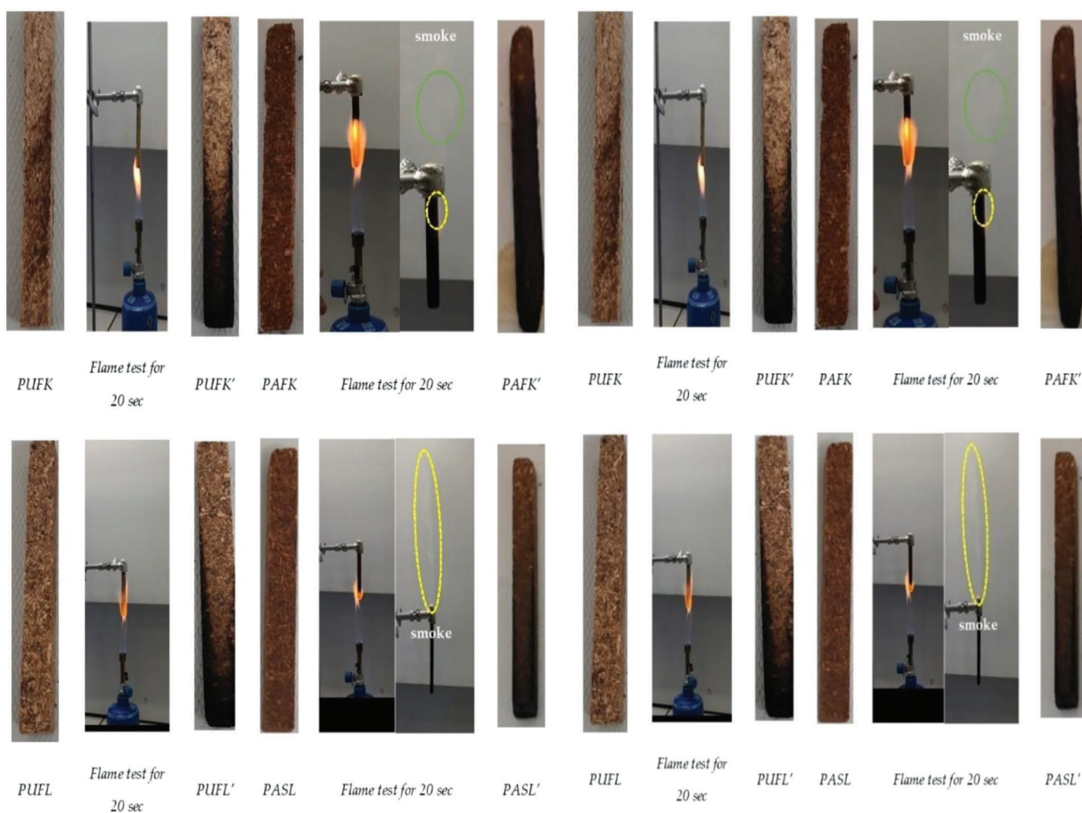
Figure 7: Particleboard before and after the vertical fire test for 20 s: ULEF-UF particleboard (PKUF), ULEF-UF particleboard with lignin (PuFL), ULEF-UF particleboard with lignosulfonate (PUFLs), ULEF-UF particleboard with lignosulfonate phosphorus (PUFLsP), citric acid-sucrose particleboard (PASK), citric acid-sucrose particleboard with lignin (PASL), citric acid-sucrose particleboard with lignosulfonate (PASLs), and citric acid-sucrose particleboard with lignosulfonate phosphorus (PASLsP)
